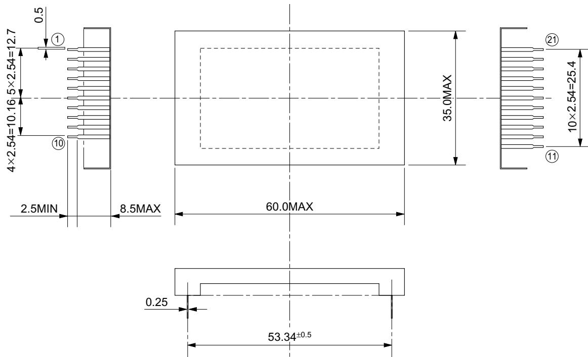
\* Dimensions are in millimeters.
