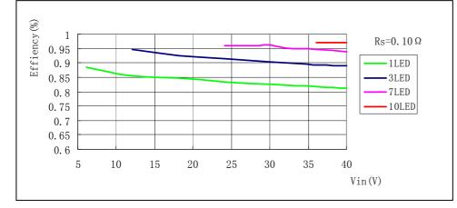
Figure 1.4 Efficiency vs. Input Supply Voltage  $(V_{IN} = 6 \text{ to } 40 \text{ V})^{\dagger}$  Per Number of LEDs (Rs=0.15 $\Omega$ , L1=47 $\mu$ H)
