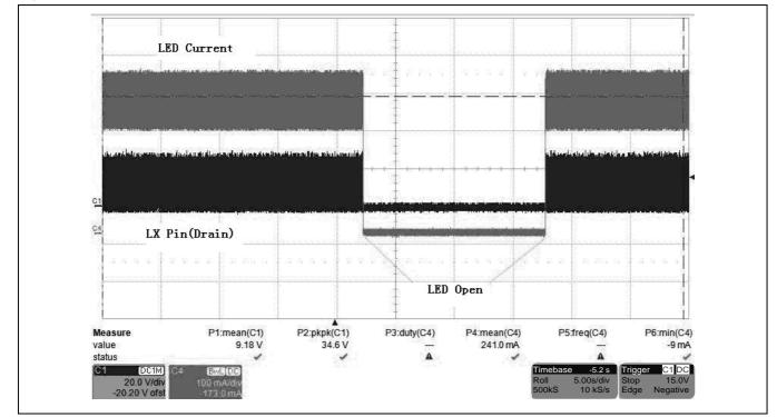
Figure 1.9 LED Open-Circuit Protection (Rs= $0.30\Omega$ , L1= $47\mu$ H, V<sub>IN</sub> = 24 V)
