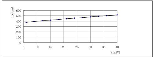
Figure 1.1 ZLED7x20 Supply Operating Current vs. Input Supply Voltage (V<sub>IN</sub> = 6 to 40 V)
