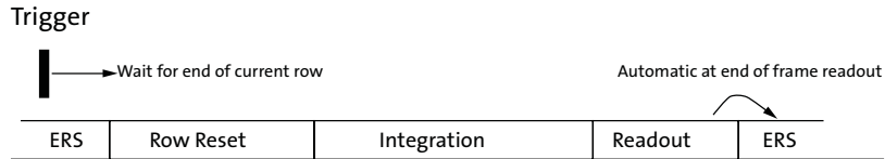
Figure 37: Entering and Leaving a Global Reset Sequence
