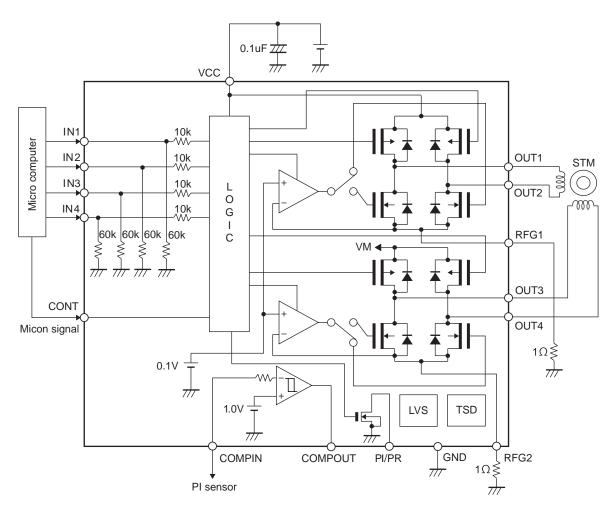
Constant-current calculation :  $I_{OUT} = 0.1 \div RF$  Example : When an  $I_{OUT}$  of 100mA is required, RF must be 1 $\Omega$ . Usage Notes
