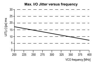
Figure 4. Maximum I/O Jitter (RMS) versus frequency for V<sub>CC</sub>=3.3V
