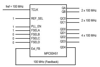
MPC93H51 zero-delay configuration (feedback of QD4)
