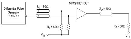
Figure 10. PCLK MPC93H51 AC test reference
