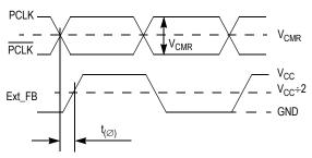
Figure 11. Propagation delay (t<sub>PD</sub>, static phase offset) test reference
