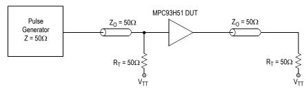
Figure 9. TCLK MPC93H51 AC test reference for V<sub>CC</sub> = 3.3V
