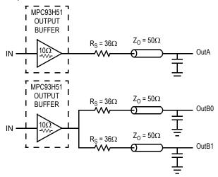
Figure 6. Single versus Dual Transmission Lines
