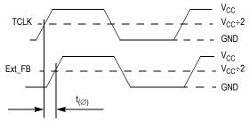
Figure 12. Propagation delay (t<sub>PD</sub>) test reference
