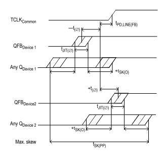
Figure 3. MPC93H51 maximum device-to-device skew
