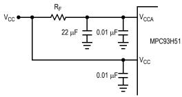
Figure 5. V<sub>CCA</sub> Power Supply Filter
