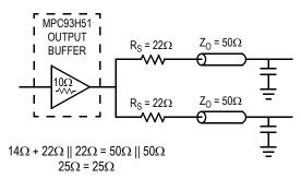
Figure 8. Optimized Dual Line Termination
