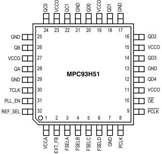
Figure 2. Pinout: 32-Lead LQFP Package Pinout (Top View)
