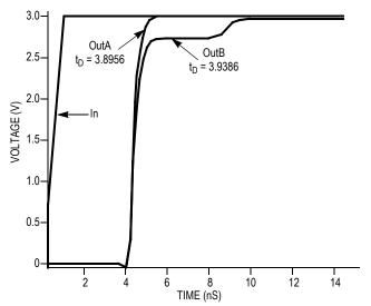
Figure 7. Single versus Dual Waveforms
