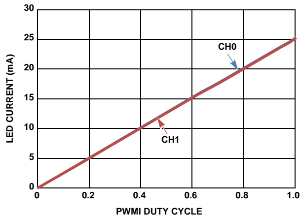
FIGURE 6. DIMMING ACCURACY (8-BIT LINEAR MODE)
