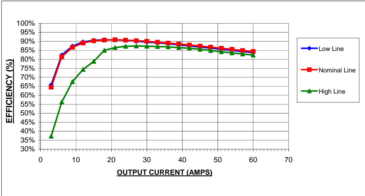
Graph 1: FA12S5-300 Efficiency vs. Output Current
