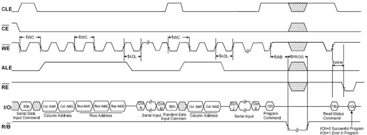
**NOTE:**  $t_{ADL}$  is the time from the  $\overline{WE}$  rising edge of final address cycle to the  $\overline{WE}$  rising edge of the first data cycle.
