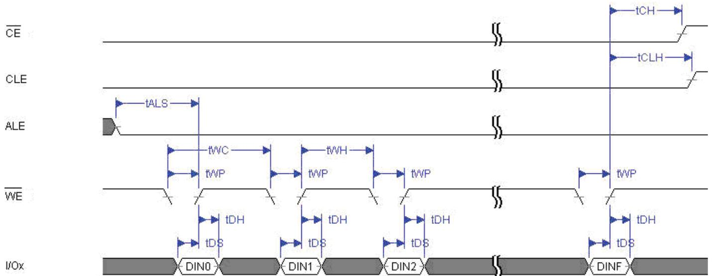
Serial Access Cycle after Read ( $CLE = L$ ,  $ALE = L$ ,  $\overline{WE} = H$ )
