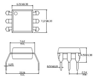
All Dimensions are in mm Tolerance = +/- 0.1mm
