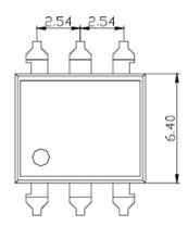
All Dimensions are in mm Tolerance = +/- 0.1mm
