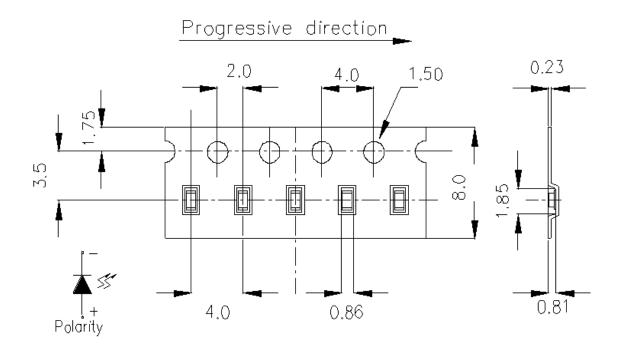
**Note:** The tolerances unless mentioned are  $\pm 0.1$  mm, unit = mm
