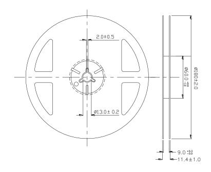
**Note:** The tolerances unless mentioned are  $\pm 0.1$  mm, unit = mm.
