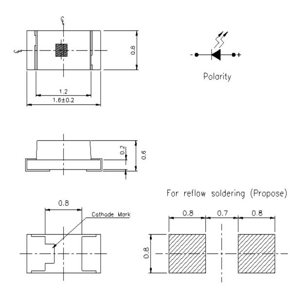
**Note:** The tolerances unless mentioned are  $\pm 0.1$  mm, unit = mm.
