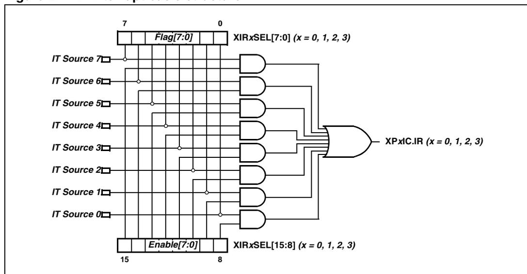
When different sources submit an interrupt request, the enable bits (Byte High of XIRxSEL register) define a mask which controls which sources will be associated with the unique available vector. If more than one source is enabled to issue the request, the service routine has to identify the real event to be serviced. This can easily be done by checking the flag
