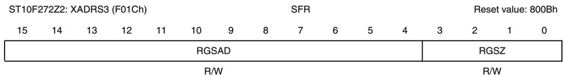
The register functionality is the same as that of ADDRSELx registers used for external address range selection, with some limitations:
