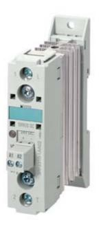
SEMICOND. CONTACTOR 3RF2, 1-PH. AC 51 10 A 40 DEGREES C 48-460 V / 24 V DC SCREW TERMINAL
