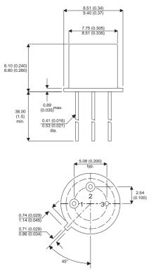
Bipolar PNP Device in a Hermetically sealed TO5 Metal Package.
