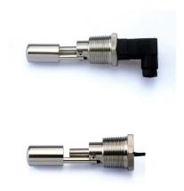
SSH66TE are externally mounted horizontal float switches with reduced length floats for applications where space is restricted. The float is of 316L Stainless Steel and the stem is of 304 Stainless Steel.
