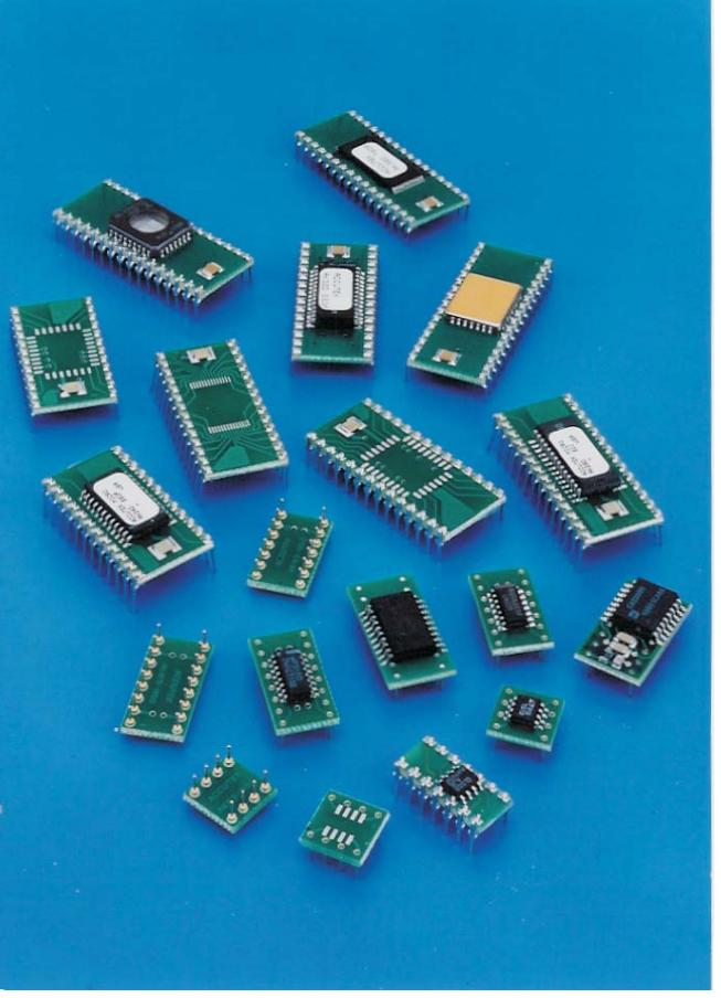
This new family of Accutek DIP Adapter Modules converts surface mount IC's to pin compatible DIP packages for creating drop-in replacements for end-of-life DIP IC's. Package types supported are: SOJ, PLCC, SOIC, SOP, TSOP, QSOP, HSOP, MSOP, LLP (Leadless Leadframe Package), CSP (Chip Scale Package) and CLCC.
