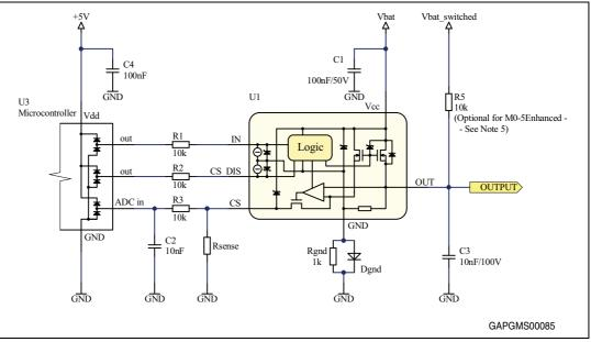
Figure 2. Monolithic analogue HSD - application schematic
