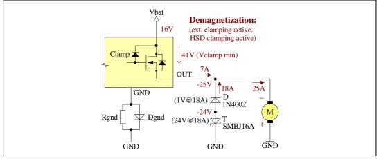
The output voltage during the demagnetization phase is -25 V (considering a worst case HSD  $V_{ClampMin}$  = 41 V,  $V_{BAT}$  = 16 V).
