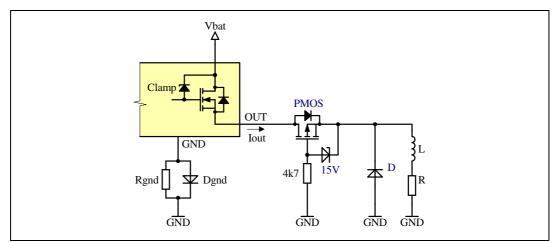
This circuitry is an improvement of the previous example. The reverse battery protection of the freewheeling diode (and load) is solved by a PMOS circuitry with negligible voltage drop at nominal current (to avoid undesired power dissipation in on-state)
