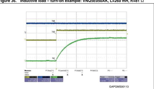
Figure 36. Inductive load – turn-on example: VNQ5E050AK, L=260 mH, R=81  $\Omega$
