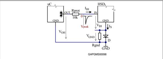
Therefore, each microcontroller I/O pin connected to a HSD must be protected by a serial resistor to limit the injected current. The value of  $R_{PROT}$  must be high enough to ensure that injected current is always below the latch-up limit of the microcontroller I/O. We should also consider the voltage drop on  $R_{PROT}$  because the current required by the HSD input is typically 10 µA. The following condition must be fulfilled:
