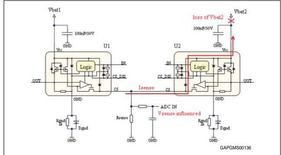
Figure 59. Direct connection of CS pins (not recommended) – Monolithic HSD
