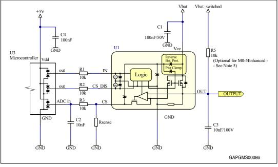
If current sense disable function is not required, CS\_DIS pin should be left open or connected to ground through a resistor (~10 kΩ). Direct connection to ground is not safe (ISO pulses clamped through CS\_DIS pin can damage the device).
