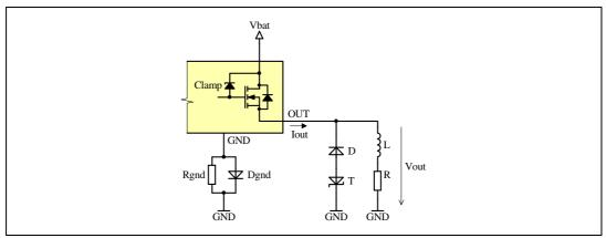
The transil (T) clamps the demagnetization voltage to a safe level. The clamping voltage of the transil should be selected in a way that the voltage across the HSD channel is below the minimum specified clamping voltage of the HSD (41 V). The diode (D) is included to protect the transil during normal operation (positive output voltage).
