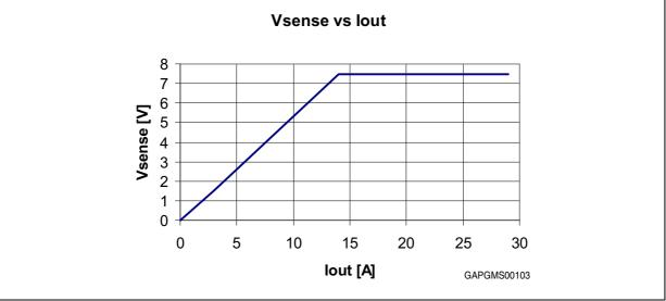
On the other hand, care must be taken to prevent the P channel MOSFET M1 from saturation, causing the I<sub>SENSE</sub> to again be disproportional with I<sub>OUT</sub>. This normally happens when the maximum current that M1 is able to supply is reached (11 mA typ.)
