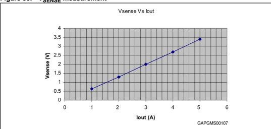
Figure 30. V<sub>SENSE</sub> measurement
