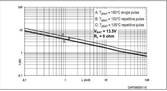
Figure 39. Maximum turn-off current versus inductance – VND5E160AJ datasheet
