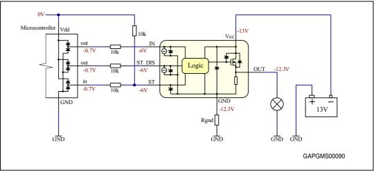
Figure 4. Voltage levels during reverse battery – resistor protection
