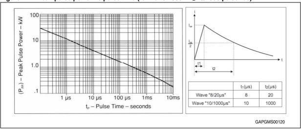
Figure 44. Peak pulse power vs pulse time (for transil 600 W@10/1000 µs series)
