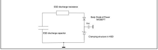
A positive ESD pulse on the output is transferred through the body diode of the power MOSFET to the Vcc pin of the HSD, so the same requirements to dimension the external capacitor apply as the negative ESD pulses on the output.
