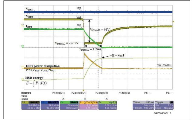
The demagnetization energy dissipated in the HSD was measured by an oscilloscope with mathematical functions. The first function (F1) shows the actual power dissipation on the HSD ( $V_{BAT} - V_{OUT}$ ) ×  $I_{OUT}$ , the second function (F4) shows the HSD energy (integral of F1).
