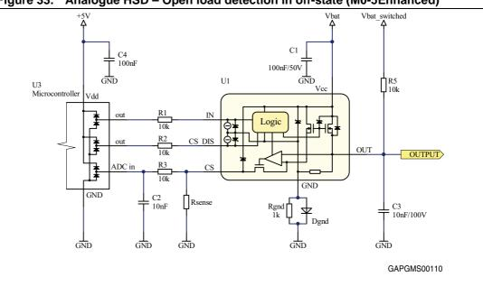
Figure 33. Analogue HSD – Open load detection in off-state (M0-5Enhanced)
