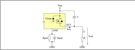
The HSD channel is protected directly by the parallel transil. The clamping voltage of the transil should be below the minimum clamping voltage of the HSD (41 V). Such transils ( $V_{CL}$  < 41 V) usually start conducting at 30 V, therefore there is a high probability that it is damaged during the clamped load dump pulse (36 V). For that reason it is usually better to use the previously described solution (1).
