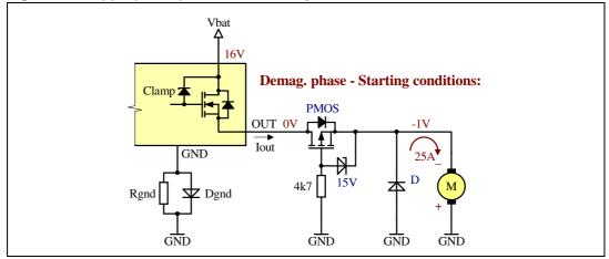
Demagnetization time - *Equation 12* (Assuming  $V_{DEMAG} = -1 V$ ) :
