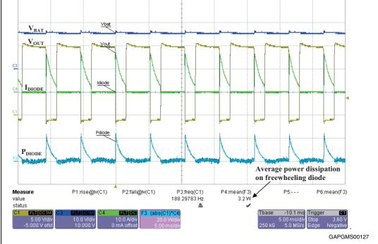
The average power dissipation measured on the freewheeling diode is 3.2 W, while the HSD thermal shutdown cycling frequency was 188 Hz. These values are below theoretical calculations. Real HSD cycling frequency is much lower than the frequency assumed in the calculation (500 Hz – based on simulation with resistive load).
