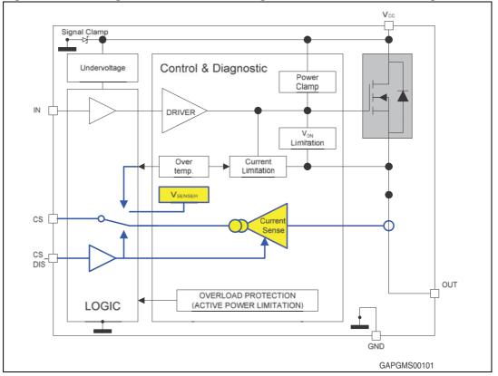
Figure 24. M0-5 High Side Driver with analogue current sense – block diagram
