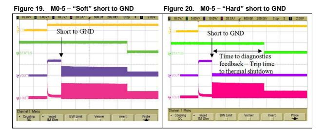
Figure 16. M0-5 – "Hard" short to GND
