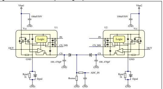
Figure 60. Safe solution for paralleling CS pins
