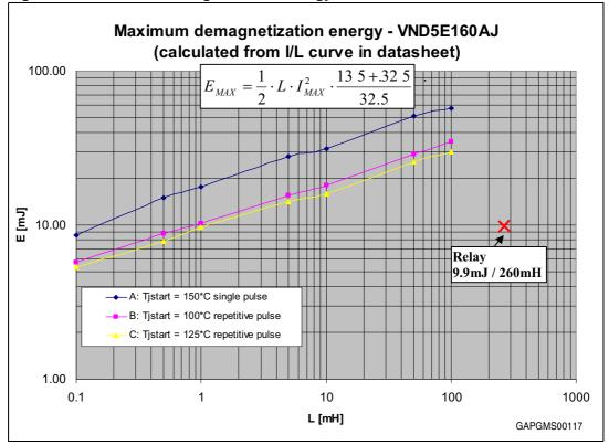
Figure 40. Maximum demagnetization energy – VND5E160A
