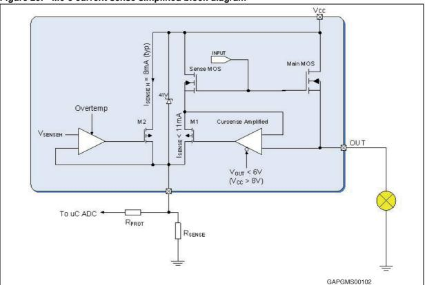
Figure 25. M0-5 current sense simplified block diagram
