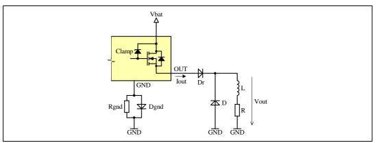
A general purpose diode connected in parallel with the load provides a conductive path for proper demagnetization. Relatively small demagnetization voltage (1 diode voltage drop in forward direction) leads to a very slow demagnetization. This can have a negative influence when driving the relay, for example. A slow movement of the armature (slow opening of contacts) can have a negative influence on the lifetime of the relay contacts (depending on the switching current).
