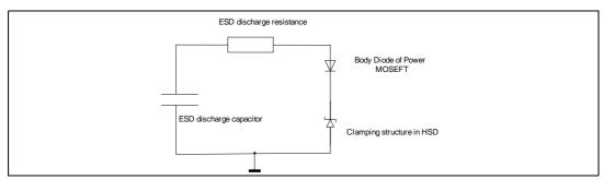
A positive ESD pulse on the output is transferred through the body diode of the power MOSFET to the Vcc pin of the HSD, stressing the Vcc-GND clamping structure. The ESD ratings of the Vcc-GND clamping structure is the same for the output clamping structure.
