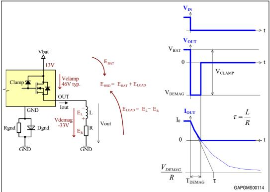
Figure 37. Inductive load – HSD turn-off phase
