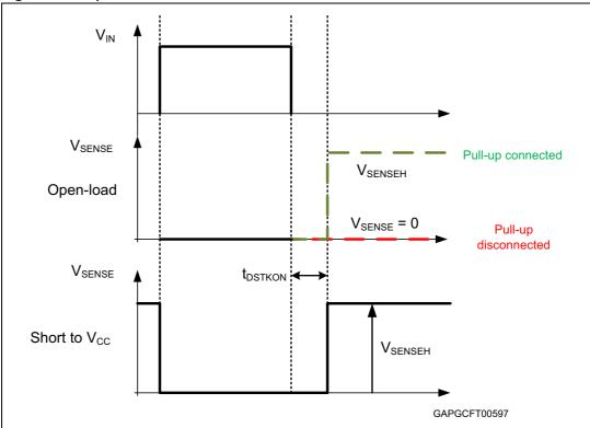
Figure 14. Open load/short to Vcc condition
