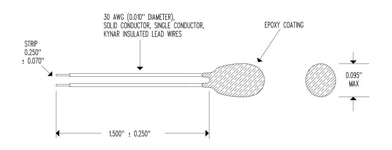
RESISTANCE @  $+25^{\circ}C = 10,000 \Omega$  NOMINAL ACCURACY (0 TO  $+70^{\circ}$ C) = ± 0.10°C RESISTANCE/TEMPERATURE CURVE = "J" TEMPERATURE COEFFICIENT @  $+25^{\circ}C = -4.4\%$ /C NOMINAL BETA " $\beta$ " (0 TO +50°C) = 3,892°K NOMINAL DISSIPATION CONSTANT = 1 mW/°C NOMINAL THERMAL TIME CONSTANT = 10 SECONDS MAXIMUM (STILL AIR)
