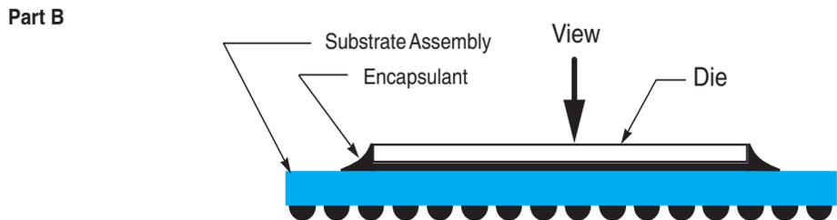
Figure 3 (in part A) shows the pinout of the PC755, 360 PBGA packages as viewed from the top surface. Part B shows the side profile of the PBGA package to indicate the direction of the top surface view.
