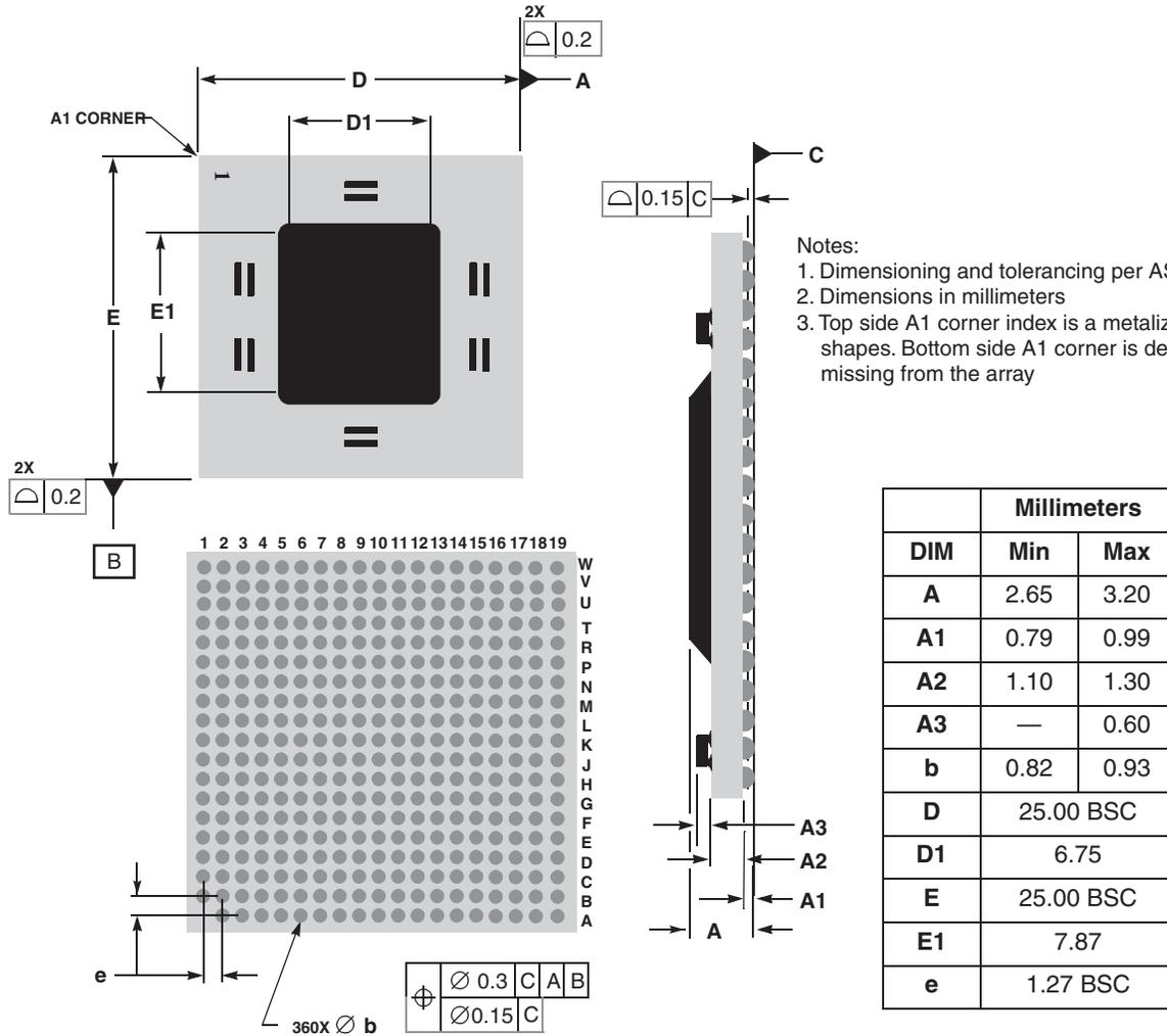
**Mechanical Dimensions of the PC755 HiTCE Package**
