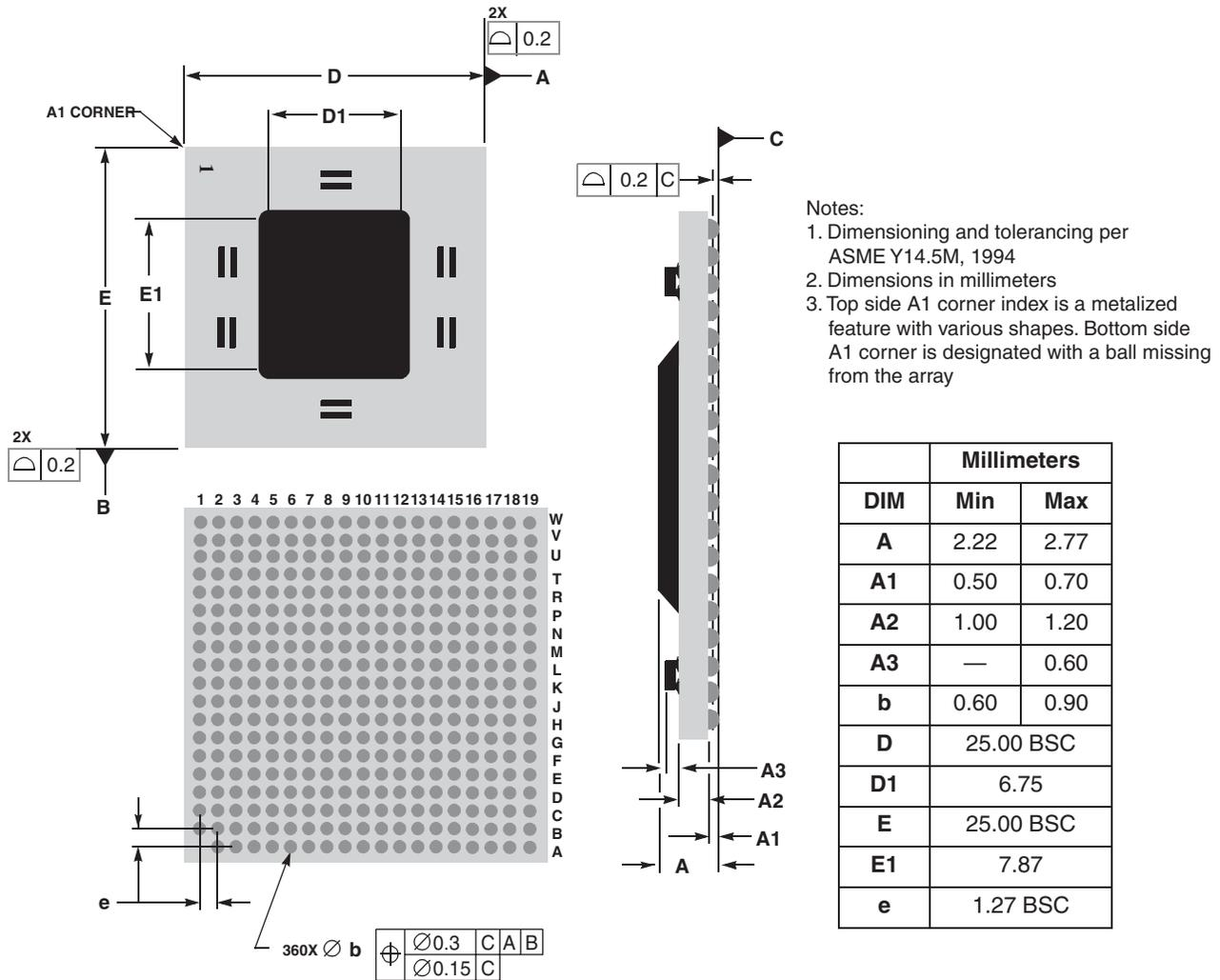
**Mechanical Dimensions of the PC755 CBGA Package**
