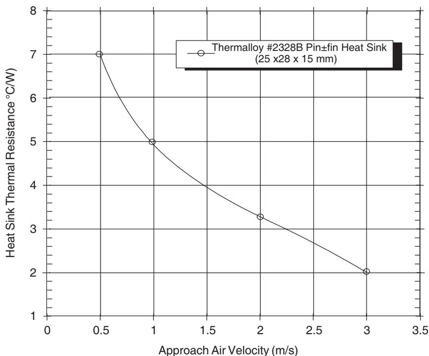
Assuming an air velocity of 0.5 m/s, we have an effective  $R_{sa}$  of 7°C/W, thus
