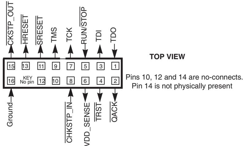
There is no standardized way to number the COP header shown in [Figure 24](#); consequently, many different pin numbers have been observed from emulator vendors. Some are numbered top-to-bottom then left-to-right, while others use left-to-right then top-to-bottom, while still others number the pins counter clockwise from pin one (as with an IC). Regardless of the numbering, the signal placement recommended in [Figure 24](#) is common to all known emulators.
