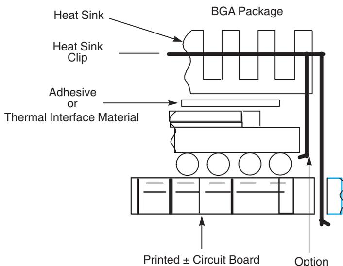
Ultimately, the final selection of an appropriate heat sink depends on many factors, such as thermal performance at a given air velocity, spatial volume, mass, attachment method, assembly, and cost.
