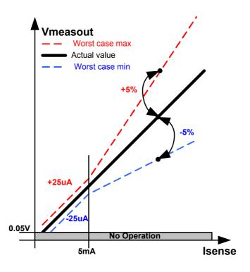
In the above graph the errors values are shown in Current Mode. Down to 5mA %Meas\_lerr1 and below 5mA IMeas\_lerr2.
