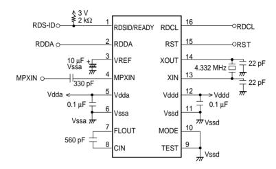
Caution: If the RST pin is unused, it must be connected to ground.
