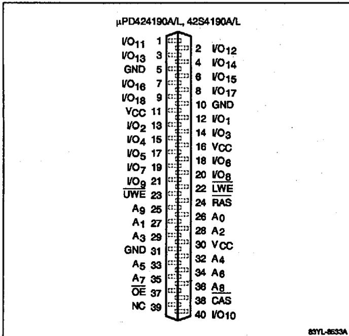
44/40-Pin Plastic TSOP (Normal Pinouts)
