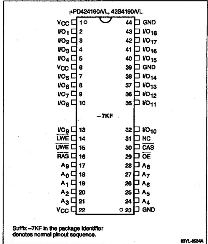
44/40-Pin Plastic TSOP (Reverse Pinouts)
