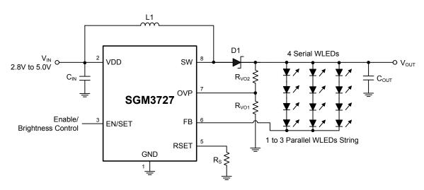
Figure 2. Application for Driving 3 × 4 WLEDs
