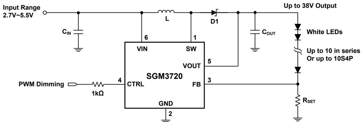
**ELECTRICAL CHARACTERISTICS (1)**(V<sub>IN</sub> = 3.6V, L = 22μH, C<sub>IN</sub> = 10μF, C<sub>OUT</sub> = 0.47μF, Full = -40°C to +85°C, typical values are at T<sub>A</sub> = +25°C, unless otherwise noted.)
