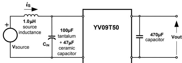
**Figure 19. Test Setup For Measuring Input Reflected-Ripple Current And Output Voltage Ripple**
