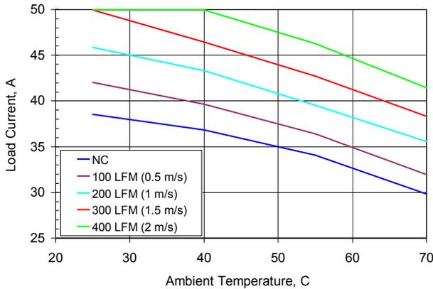
**Figure 14.** Output Current versus Local Ambient Temperature and Airflow ( $V_{in} = 12.0$  Vdc,  $V_o = 2.5$  Vdc).
