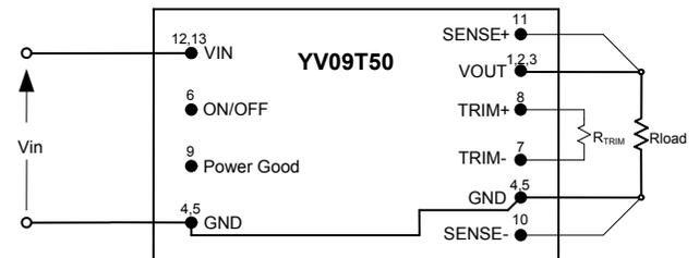
**Figure 16.** Programming Output Voltage With A Resistor
