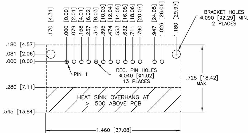
**Figure 21. Recommended Footprint – Top View**
