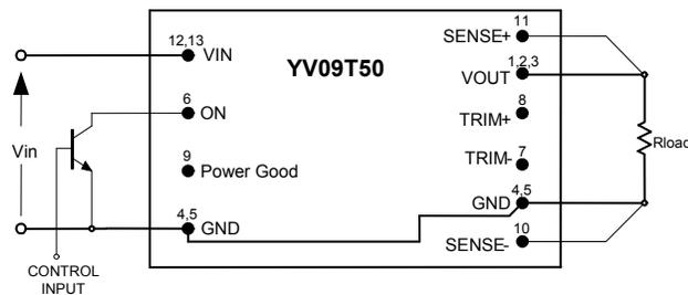
**Figure 17. Circuit Configuration For ON/OFF Function**
