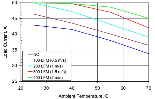
**Figure 11 Output Current versus Local Ambient Temperature and Airflow (Vin = 12.0 Vdc, Vo=0.6Vdc)**
