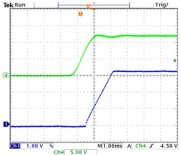
**Figure 8. Typical Start-Up with application of  $V_{in}$**
