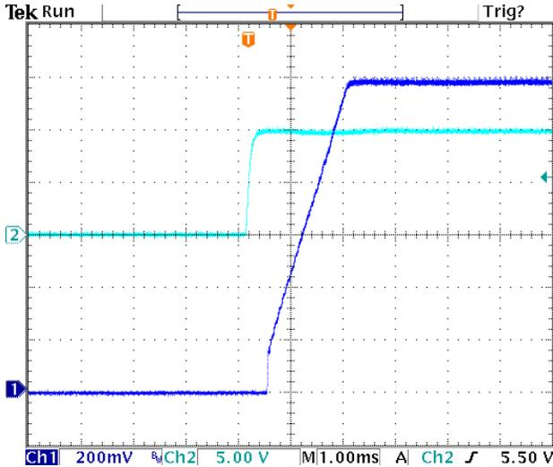
**Figure 5. Typical Start-Up Using Remote On/Off**
