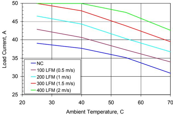
**Figure 13** Output Current versus Local Ambient Temperature and Airflow ( $V_{in} = 12.0$  Vdc,  $V_o = 1.8$  Vdc).
