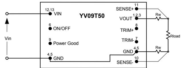
**Figure 18. Remote Sense Circuit Configuration**
