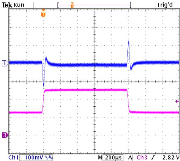
**Figure 10. Transient Response to Dynamic Load Change from 50% to 100% of full load (Vin=12V, Vo=3.3Vdc). Ch3 – Iout**
