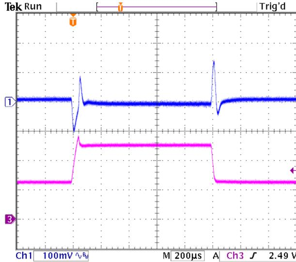
**Figure 9. Transient Response to Dynamic Load Change from 50% to 100% of full load (Vin=12V, Vo=0.6Vdc). Ch3 – Iout**
