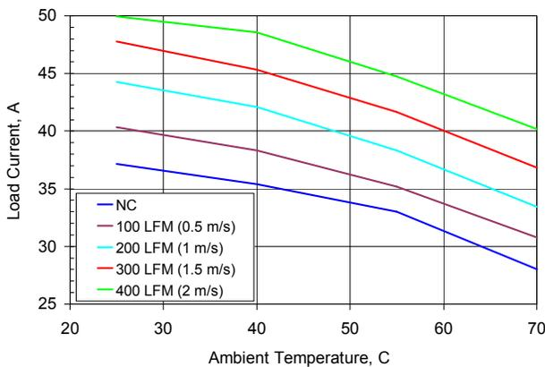
**Figure 15.** Output Current versus Local Ambient Temperature and Airflow ( $V_{in} = 12.0$  Vdc,  $V_o = 3.3$  Vdc).
