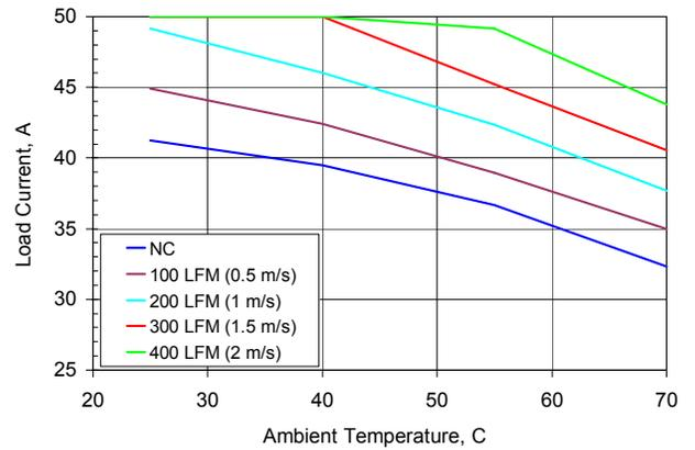
**Figure 12. Output Current versus Local Ambient Temperature and Airflow (Vin = 12.0 Vdc, Vo=1.2Vdc).**
