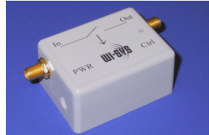
The WS2803 is a general-purpose, high performance, high isolation solid-state L-Band and S-Band RF coaxial switch. The high switching speed also allows for the user to send bursts of RF signal, making it suitable for testing RF detectors, power regulated amplifiers or any other devices operated under rapidly varying RF levels.
