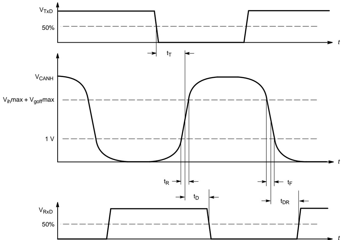
**Figure 3. Input/Output Timing**
