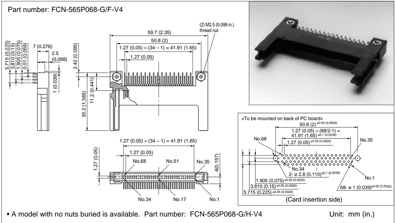
**RIGHT-ANGLE PLUG, THROUGH-HOLE TYPE (WITH NO EJECTOR, RAISED MOUNTING TYPE) SUPPORTS TYPE I, II CARDS**
