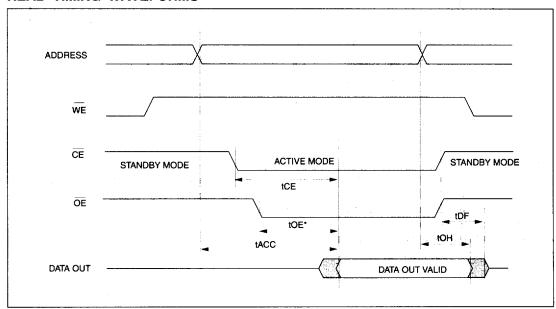
\* If  $\overline{\sf CE}$  is kept low and address pins are kept at constant during power-up, the time period between  $\overline{\sf OE}$  going low and data out valid shoul be treated as tACC instead of tOE.
