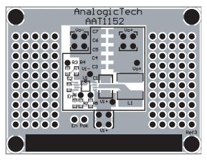
Figure 2. AAT1152 Evaluation Board PCB Top Side.
