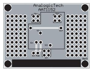
Figure 3. AAT1152 Evaluation Board PCB Bottom Side.
