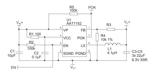
Figure 1: AAT1152 Evaluation Board Schematic.
