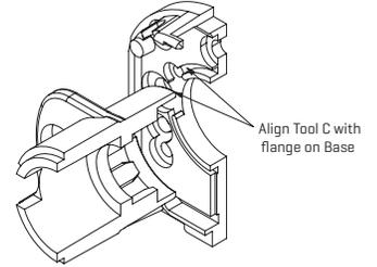
1. Align Tool C with flange on Base.
