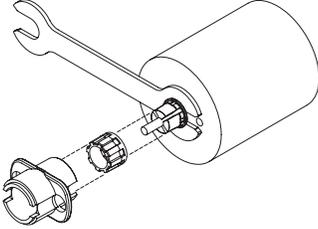
1. Insert Tool A as a spacer that defines the distance to the mounting surface.
