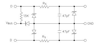
Figure 2 - STF203-22 Connection Diagram (Full Speed Devices)
