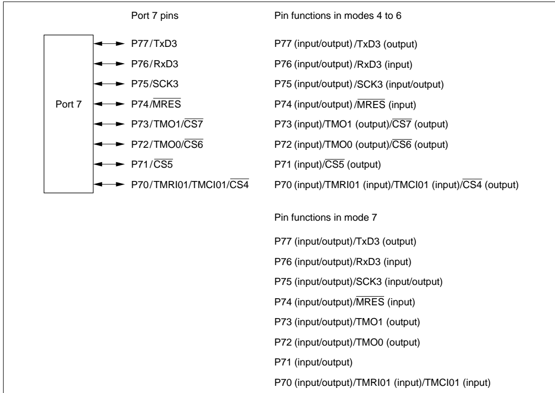
Figure 9-4 Port 7 Pin Functions
