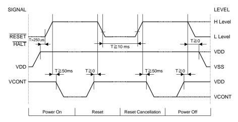
Please maintain the above sequence when turning on and off the power supply of the module. If  $V_{EE}$  and/or  $V_{CONT}$  is supplied to the module while internal alternate signal for LCD driving (M) is unstable or  $\overline{RESET}$  and  $\overline{HALT}$  is active, DC component will be supplied to the LCD panel. This may cause damage to the LCD module.
