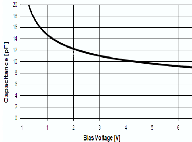
Figure 3. Filter Capacitance vs. Input Voltage (Normalized to Capacitance at 0 VDC and 25°C)
