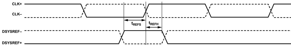
Figure 3. DSYSREF+/DSYSREF- Setup and Hold Timing (Clock Divider = 1)
