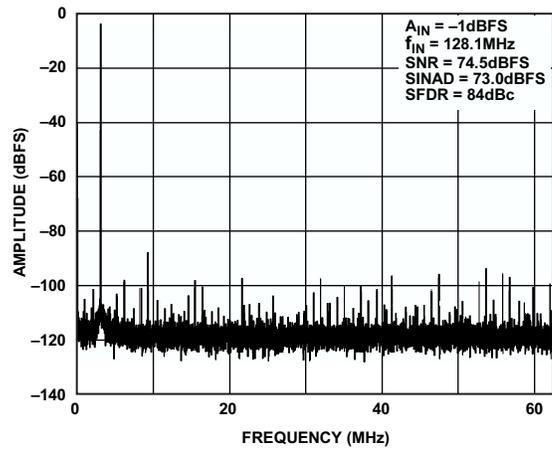
Figure 24. Single-Tone 32k FFT with  $f_{IN} = 128.1\text{ MHz}$ ,  $f_{SAMPLE} = 125\text{ MSPS}$ ,  $V_{REF} = 1.0\text{ V}$
