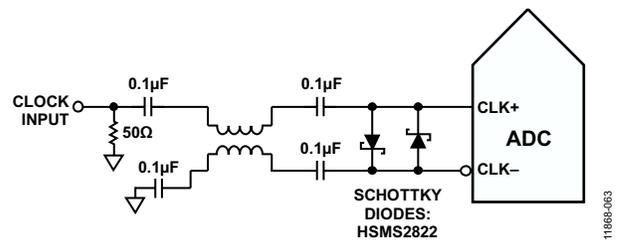
Figure 57. Balun-Coupled Differential Clock (Up to 1 GHz)
