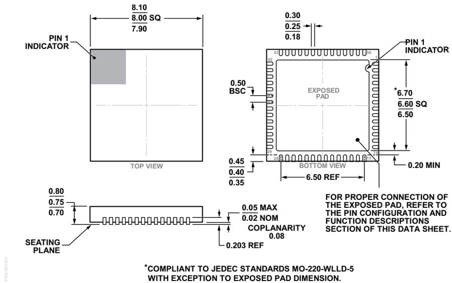
*Figure 71. 56-Lead Lead Frame Chip Scale Package [LFCSP\_WQ]
