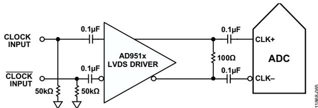
Figure 59. Differential LVDS Sample Clock (Up to 1 GHz)
