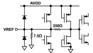
Figure 44. Equivalent VREF Circuit
