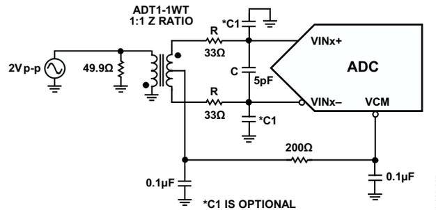
Figure 49. Differential Transformer-Coupled Configuration for Baseband Applications
