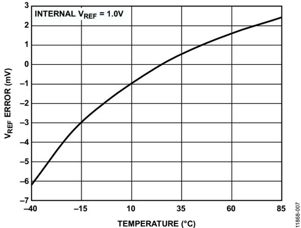
Figure 54.  $V_{REF}$  Error vs. Temperature, Typical  $V_{REF} = 1.0$  V Drift
