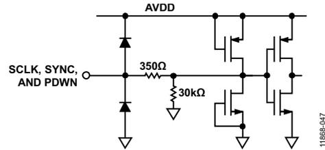
Figure 41. Equivalent SCLK, SYNC, and PDWN Input Circuit
