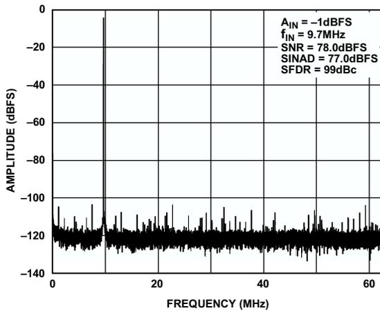
Figure 21. Single-Tone 32k FFT with  $f_{IN} = 9.7\text{ MHz}$ ,  $f_{SAMPLE} = 125\text{ MSPS}$ ,  $V_{REF} = 1.0\text{ V}$
