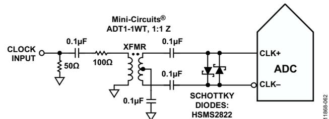
Figure 56. Transformer-Coupled Differential Clock (Up to 200 MHz)
