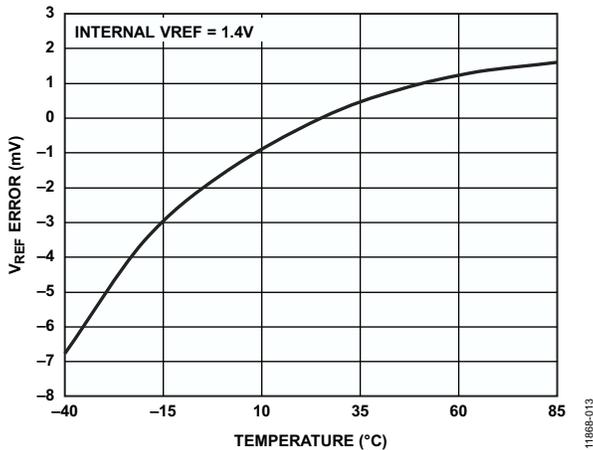
Figure 55.  $V_{REF}$  Error vs. Temperature, Typical  $V_{REF} = 1.4$  V Drift
