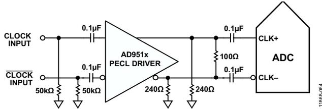
Figure 58. Differential PECL Sample Clock (Up to 1 GHz)
