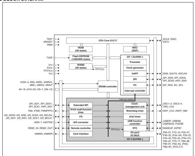
The pins enclosed in brackets () are available only for the TQFP15-128pin package model. (They are not provided in the TQFP14-100pin package model.)
