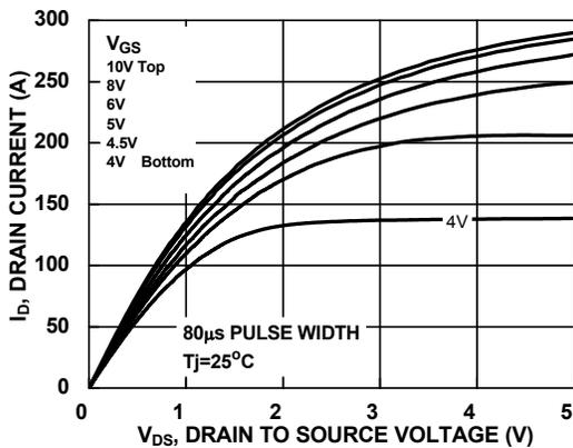
Figure 9. Saturation Characteristics
