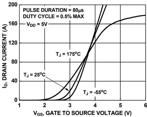
Figure 7. Transfer Characteristics
