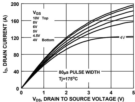
Figure 10. Saturation Characteristics
