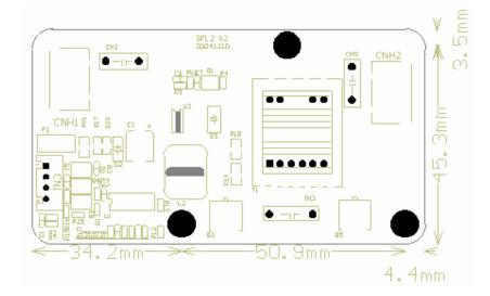
Outline: 89.5\*48.8\*9.1mm Top layer High (Max): 7.5mm Board Thickness: 1.6mm
