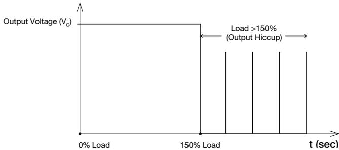
Additionally, if the  $I_o$  is  $<150\%$  but  $>100\%$  for a prolonged period of time (depending on the load), the Over Temperature Protection (OTP) will be activated due to high temperature on critical components. The power supply will then go into "Hiccup mode" until the fault is removed.
