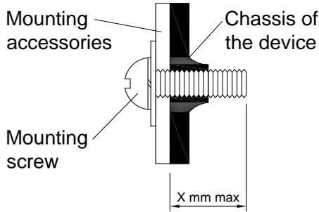
■ Only use M3 screw  $\leq X$  mm through the base mounting holes (Refer to the Screw Protrusion Length in the table below). This is to keep a safe distance between the screw and internal components.
