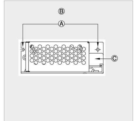
Fig. 2.3 Side Mounting (Horizontal)
