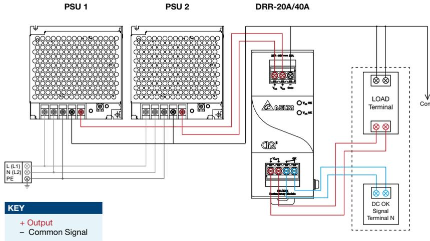
Fig. 3.1 Redundancy / Parallel Operation Connection Diagram
