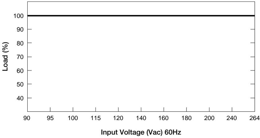
■ No output power de-rating for the input voltage from 90Vac to 264Vac
