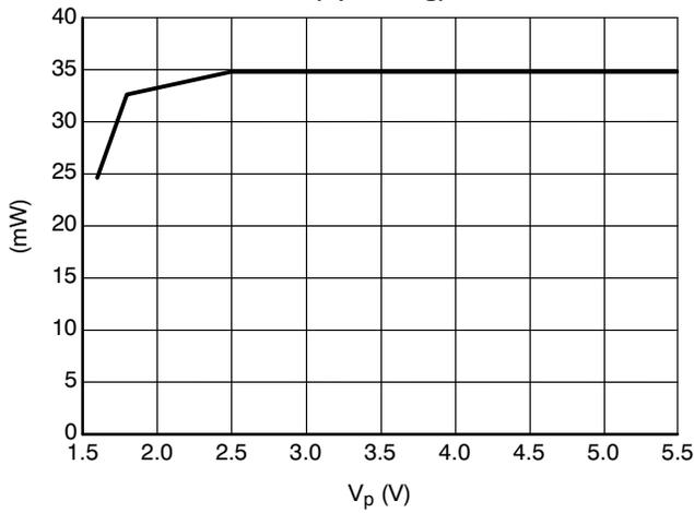
Figure 10. Maximum Output Power vs  $V_p$
