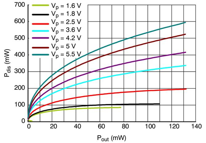
Figure 9. Power Dissipation vs  $P_{out}$  @ 25°C
