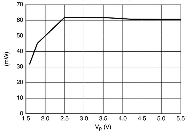
Figure 11. Maximum Output Power vs  $V_p$
