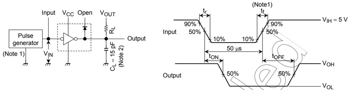
Note 1: Pulse width 50  $\mu$ s, duty cycle 10%, output impedance 50  $\Omega$ ,  $t_r \leq 5$  ns,  $t_f \leq 10$  ns
