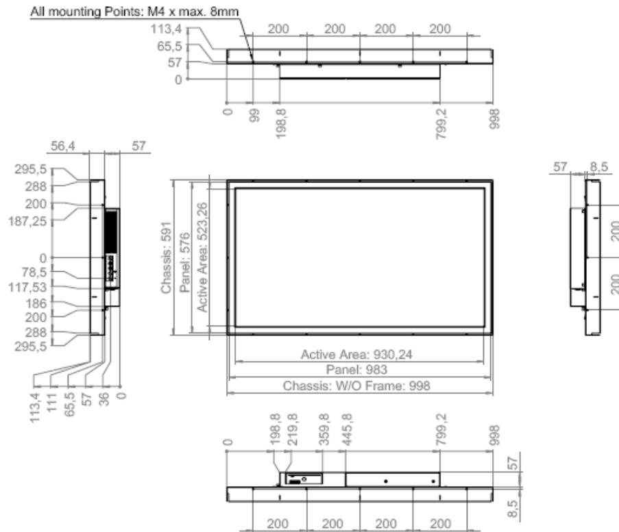
Dimensions in mm, Tolerance: DIN 2768-1 mittel
