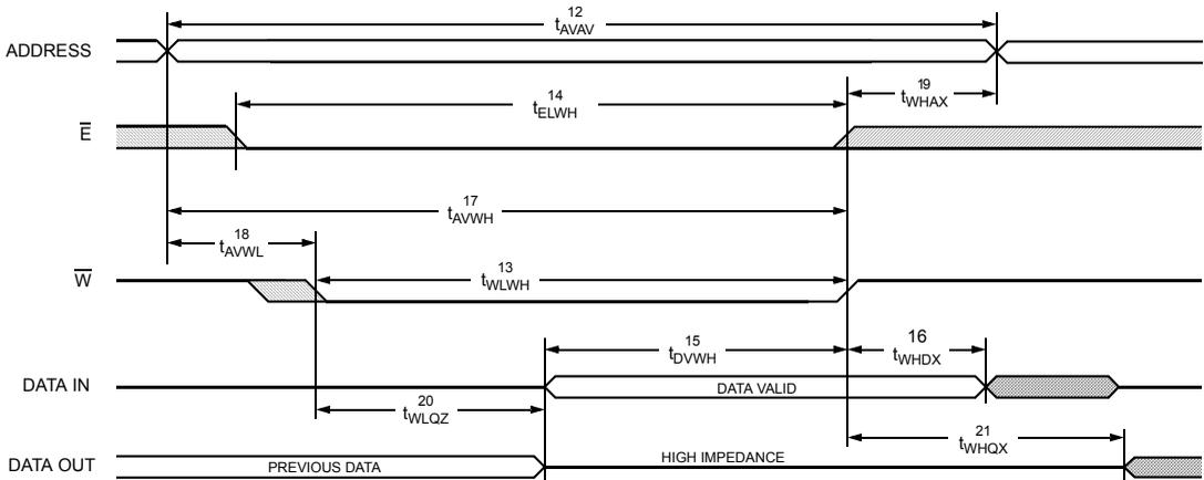
SRAM WRITE CYCLE #2:  $\bar{E}$  Controlled<sup>j</sup>
