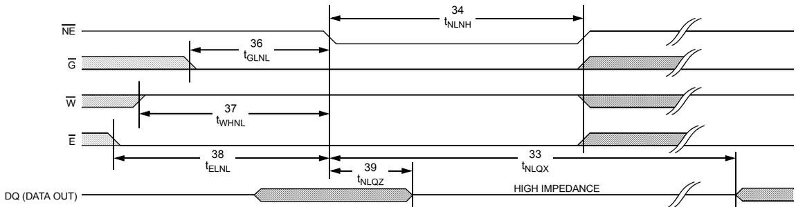
RECALL CYCLE #2:  $\overline{E}$  Controlled<sup>n</sup>
