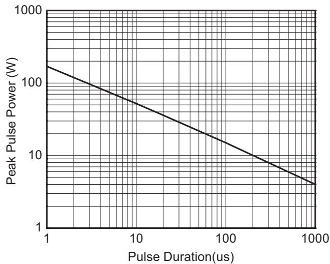
Non-Repetitive Peak Pulse Power vs. Pulse time
