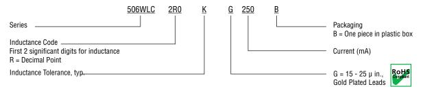
The above part number refers to a 506WLC Series 2.0 µH inductor, K tolerance (±10%, typ.), with Gold Plated Leads (G), 250 mA, one piece in plastic box.
