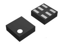
The DFN(PLP)package is a leadless package using an electroforming sheet in place of lead frame. This extremely compact package features increased power dissipation and conversion to thinner type. The name is representing by a combination of the body size and the number of pins, i.e., DFN(PLP)1212-6 stands for the body size of 1.2mm×1.2mm and 6pins.
