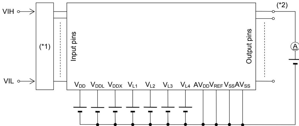
\*1: Input logic circuit to determine the specified measuring conditions.
