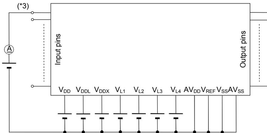
\*3: Measured at the specified output pins.
