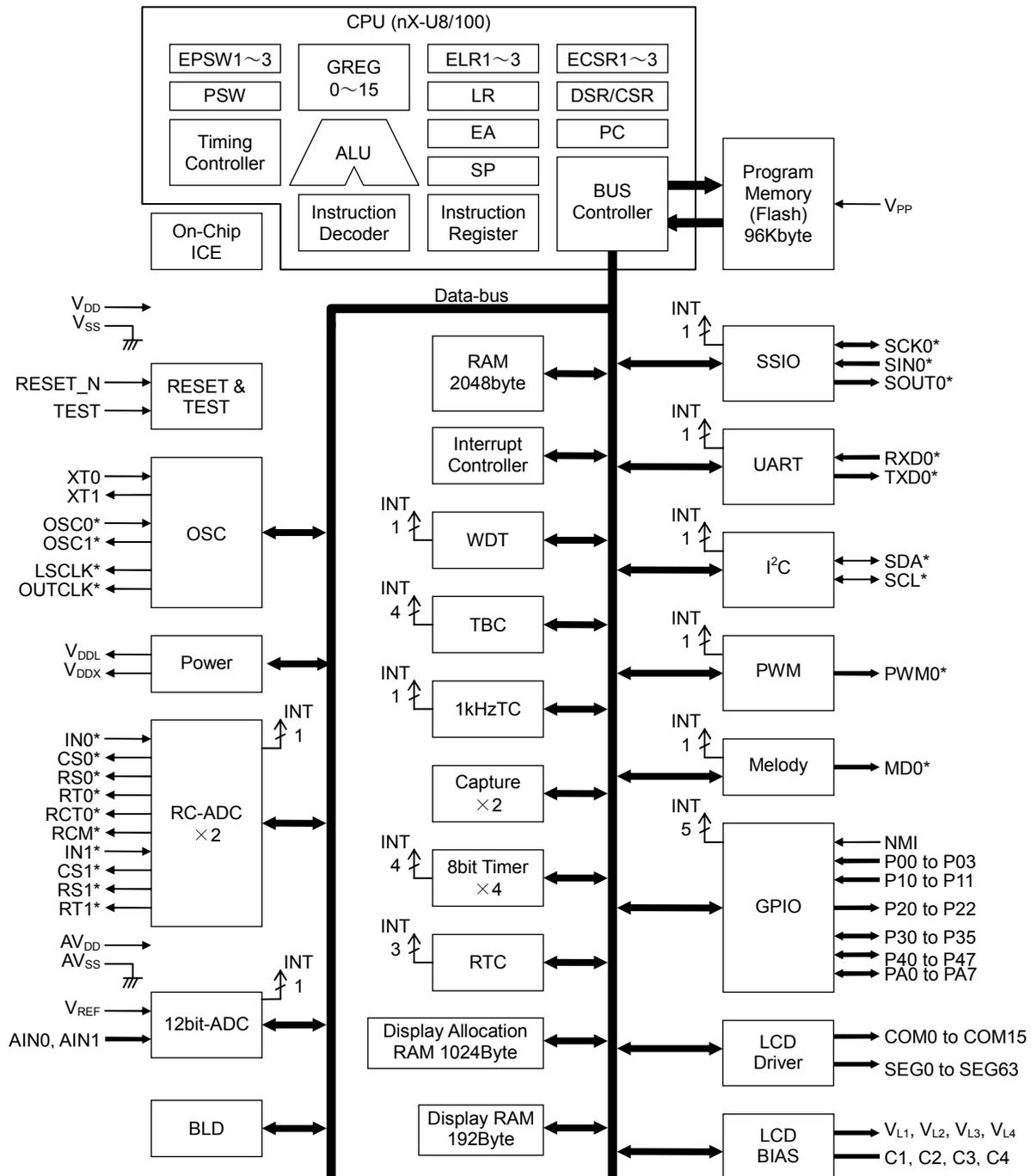
Figure 1 ML610Q435 Block Diagram
