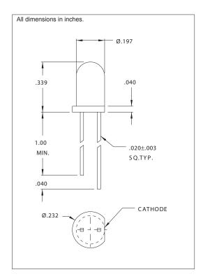
These T-1 3/4 LED lamps contain an integral resistor in series with the emitter chip to allow their direct application into 5 and 12 volt circuits. No external current limiting resistor is required. These lamps allow for savings in both component and assembly cost. These LEDs are compatible with all conventional soldering techniques.
