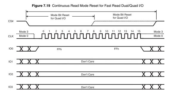
Since S25FL008K does not have a hardware Reset pin, so if the controller resets while S25FL008K is set to Continuous Mode Read, the S25FL008K will not recognize any initial standard SPI instructions from the controller. To address this possibility, it is recommended to issue a Continuous Read Mode Reset instruction as the first instruction after a system Reset. Doing so will release the device from the Continuous Read Mode and allow Standard SPI instructions to be recognized.
