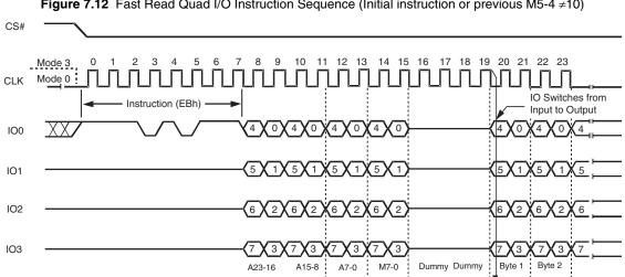
Figure 7.12 Fast Read Quad I/O Instruction Sequence (Initial instruction or previous M5-4 ≠10)
