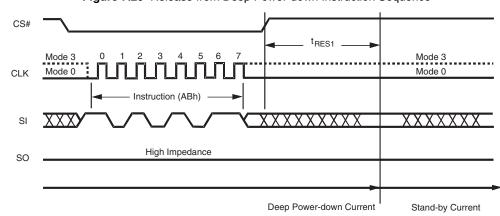
Figure 7.29 Release from Deep Power-down Instruction Sequence
