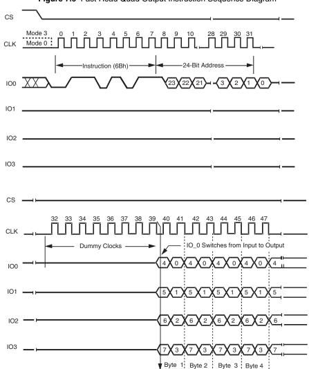
Figure 7.9 Fast Read Quad Output Instruction Sequence Diagram
