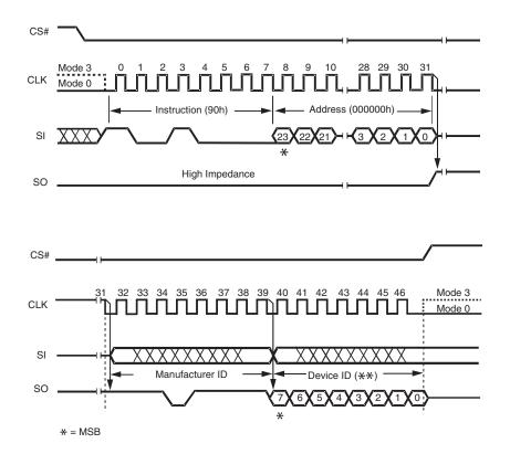
Figure 7.31 Read Manufacturer / Device ID Diagram
