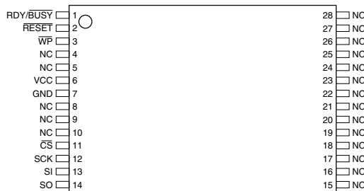
TSOP Top View Type 1
